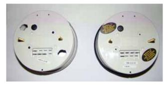
AutoMeter 5 inch Series I and Series II tachometers (left) and speedometers (right) have a LAMP terminal in the 8 cavity gauge connector. Series II gauges (on the right) require the light power lead to be on this terminal. Series I gauges (on the left) use separate light sockets and the LAMP terminal is not functional. Refer to the enclosed light socket connection photo to connect these sockets.
