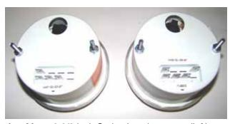
AutoMeter 3 3/8 inch Series I tachometers (left) and speedometers (right) are lit with a twist in light socket. The lamp power connection is made within the 8 cavity gauge connector on the LAMP terminal.
