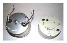
AutoMeter Mechanical speedometers will only require light socket connections. Refer to the enclosed light socket connection photo to connect these sockets.
